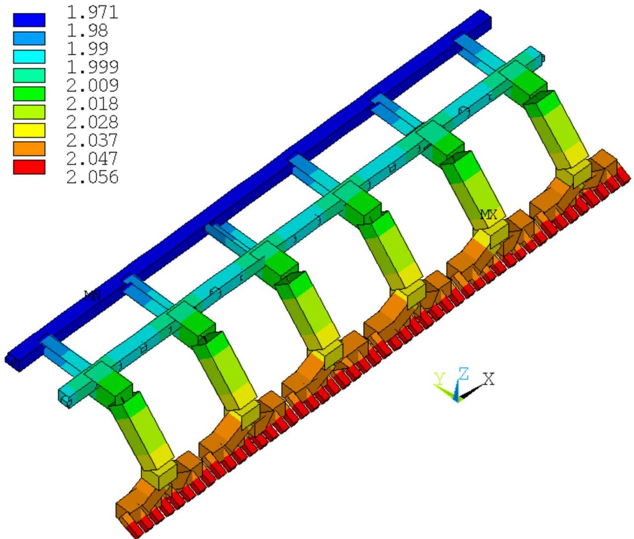
Figure 10: 520 kA 6 risers 100% downstream current extraction cell with ECC busbar network predicted voltage drop
