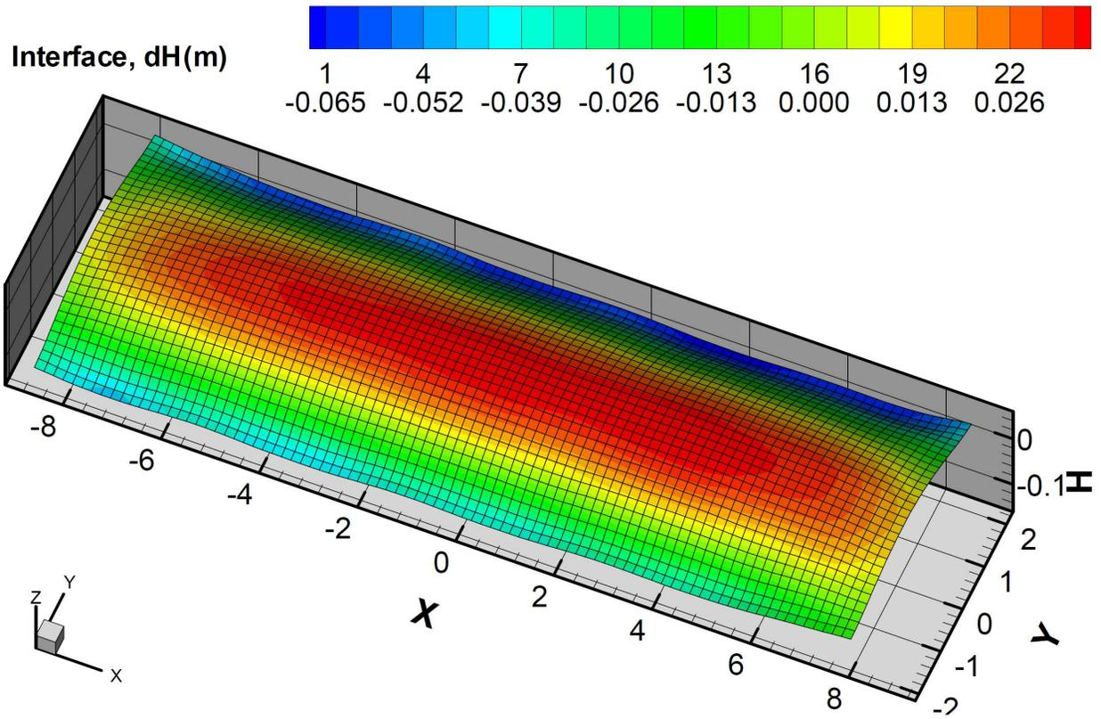
Figure 7: Wider 650 kA 8 risers RCC busbar network MHD-Valdis model bath-metal interface prediction
