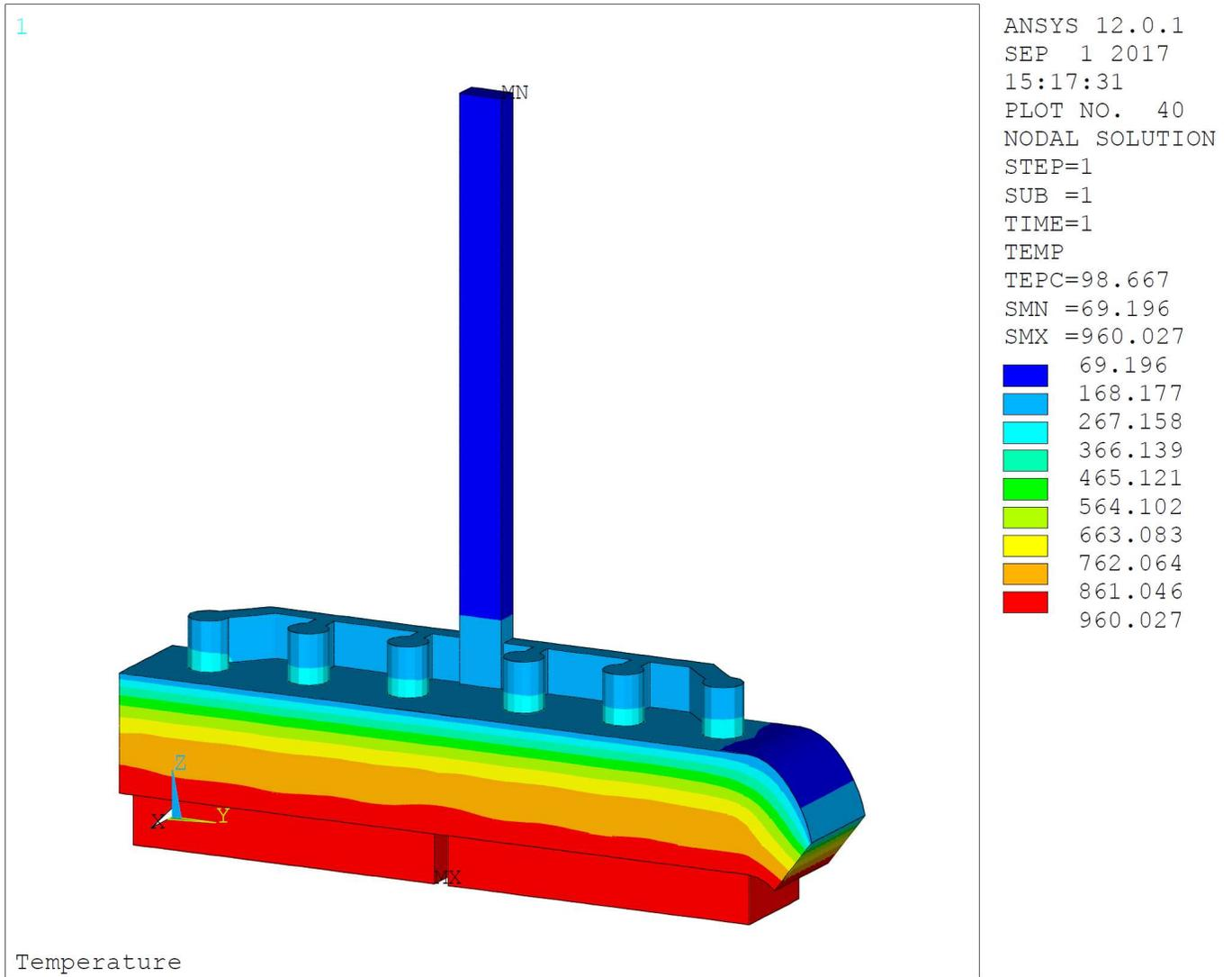
Figure 3: Anode model temperature solution
