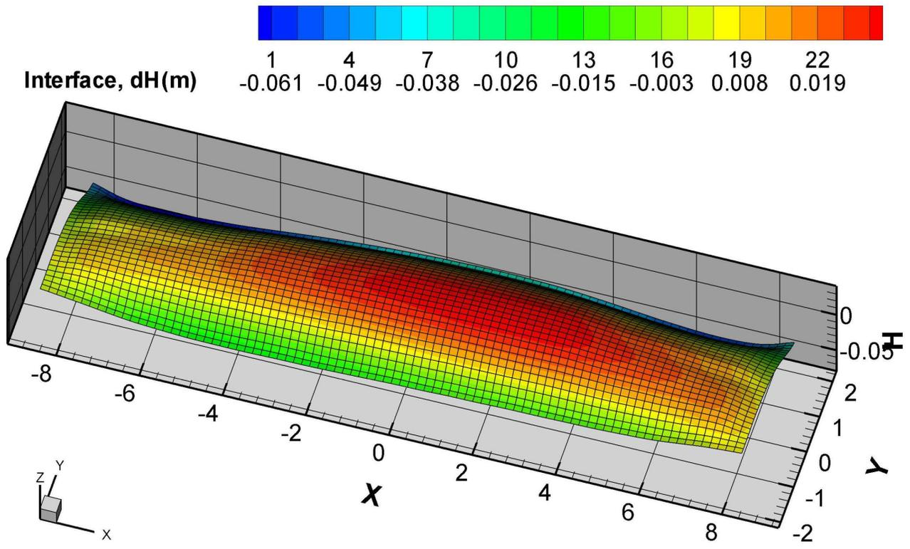
Figure 12: 520 kA 6 risers 100% downstream current extraction cell with ECC busbar network predicted bath-metal interface
