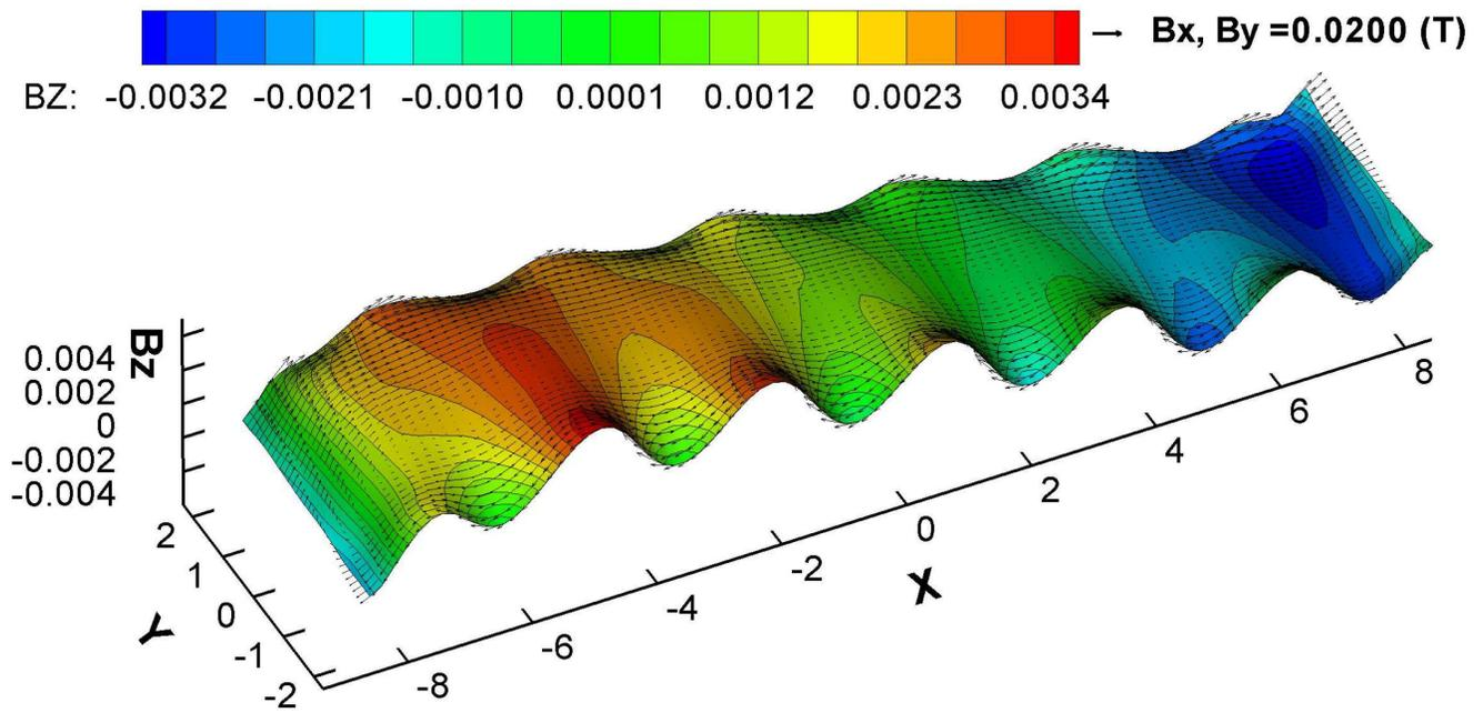
Figure 11: 520 kA 6 risers 100% downstream current extraction cell with ECC busbar network predicted BZ
