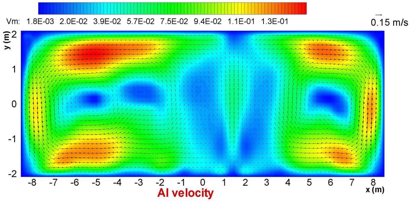
Figure 13: 520 kA 6 risers 100% downstream current extraction cell with ECC busbar network predicted metal flow field
