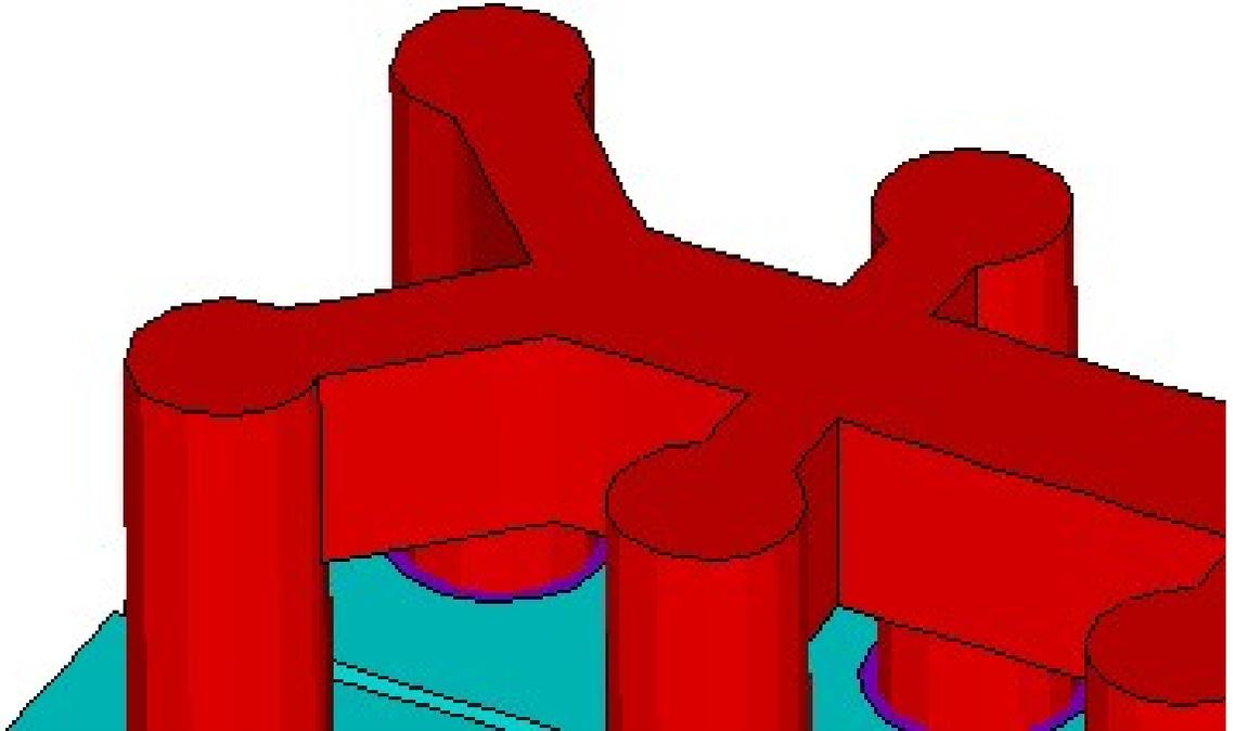
Figure 1: Topology of the 4 carbon blocks per anode, 3 stubs per carbon block new anode design
