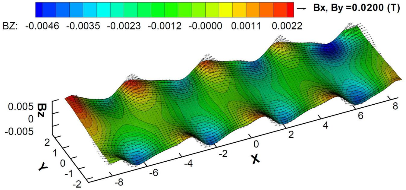
Figure 6: Wider 650 kA 8 risers RCC busbar network MHD-Valdis model  $B_z$  prediction
