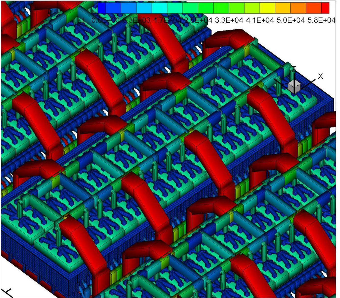
Figure 5: Wider 650 kA 8 risers RCC busbar network MHD-Valdis model setup
