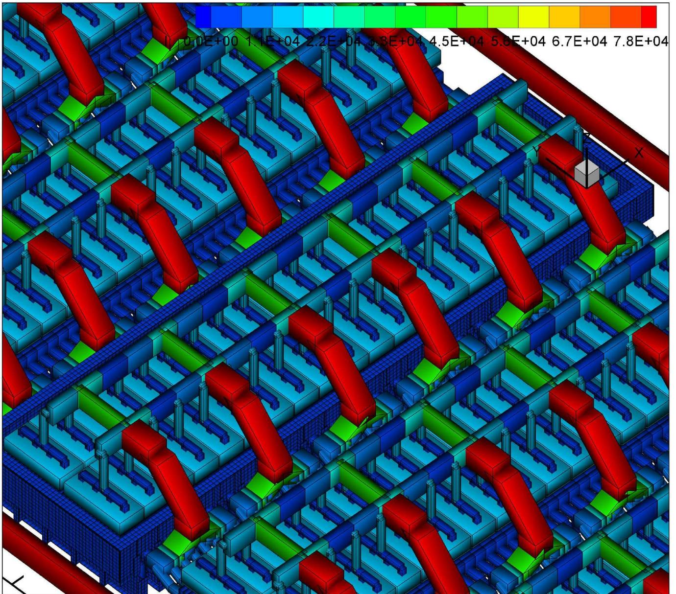
Figure 9: 520 kA 6 risers 100% downstream current extraction cell with ECC busbar network, MHD-Valdis model setup
