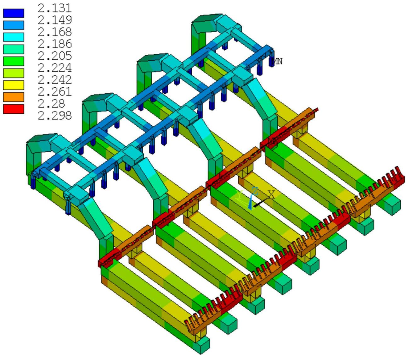
Figure 4: Wider 650 kA model predicted busbar voltage drop
