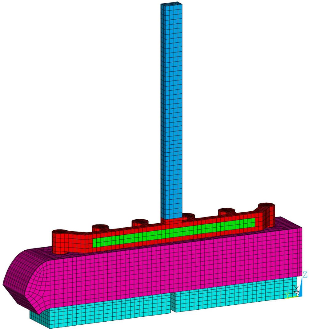
Figure 2: Half anode model mesh showing the copper insert in green
