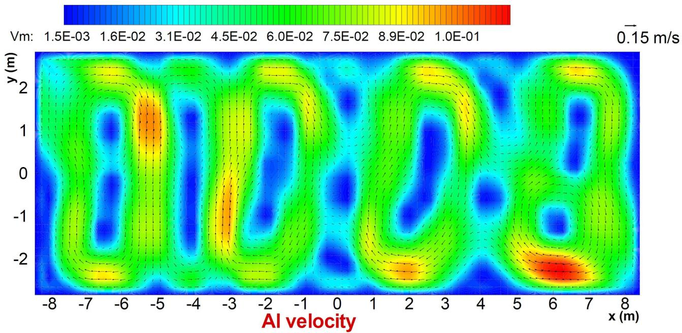
Figure 8: Wider 650 kA 8 risers RCC busbar network MHD-Valdis model metal flow field prediction
