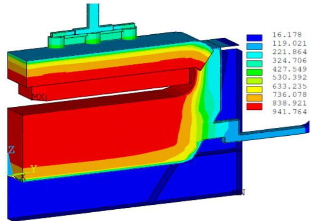
Figure 13: A697 full cell slice model temperature solution using the modified calcium silicate property
