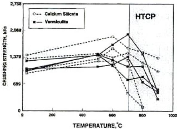
Figure 9: Observed degradation of insulating material properties above about 700 °C from [11]
