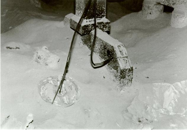
Figure 1: Measurement of the heat flux on the crust and the anode yoke using heat flux probes from Japan in the 70's
