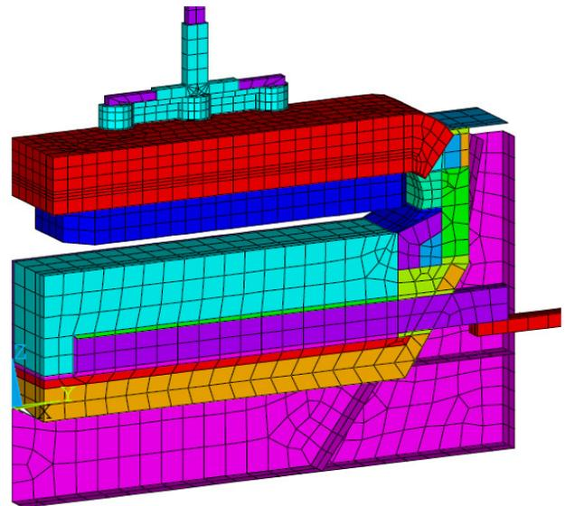
Figure 6: A697 full cell slice model mesh used in this study
