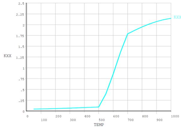
Figure 12: Temperature dependent thermal conductivity of calcium silicate material used in cell lining
