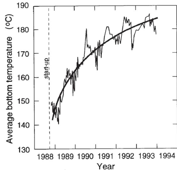
Figure 17: Averaged measured change of the potshell floor temperature of 16 155 kA prebaked cells, Figure 17 of [4]
