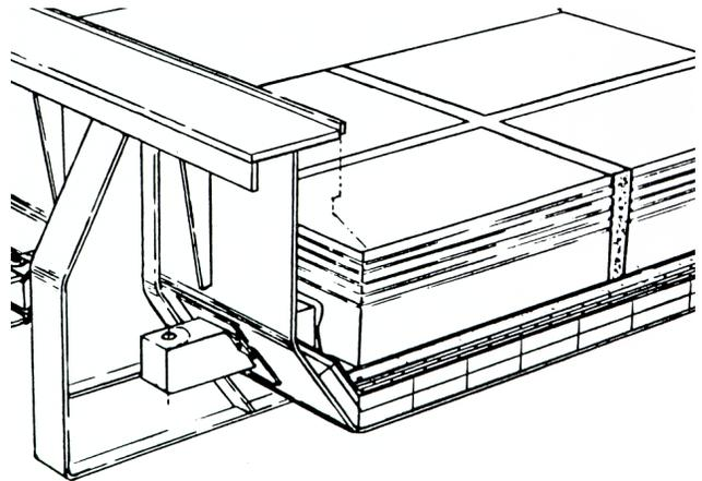
Figure 3: Original lining design of the Alcoa P155 cell, Figure 1 in [10]
