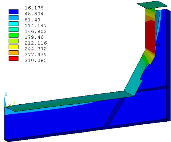
Figure 16: Potshell temperature solution using the modified calcium silicate property
