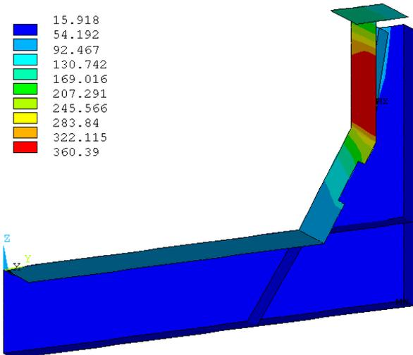
Figure 15: Potshell temperature solution using new calcium silicate property
