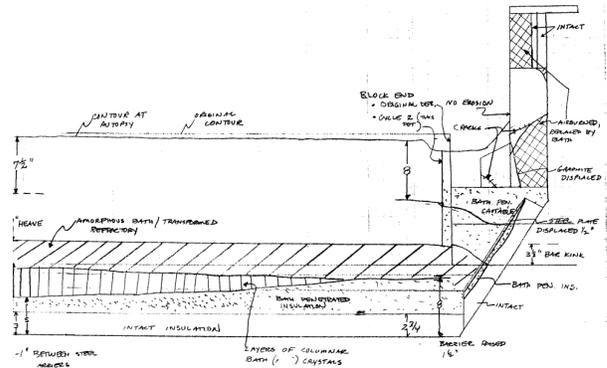
Figure 11: Sketch from a A697 cell autopsy describing the chemical degradation of the insulation layer from [8]
