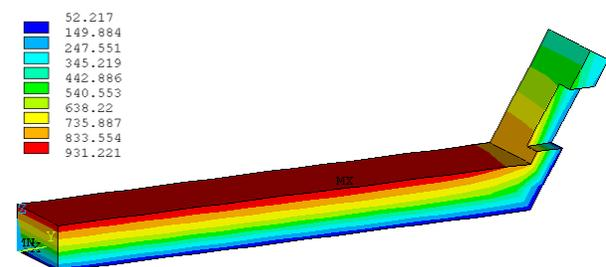
Figure 8: Calcium silicate temperature solution using new calcium silicate property
