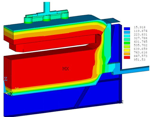
Figure 7: A697 full cell slice model temperature solution using new calcium silicate property
