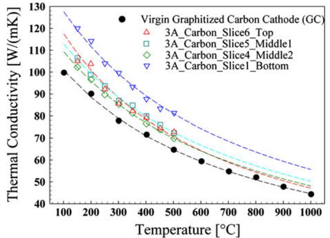
Figure 2: Example of thermal conductivity of spent cathode blocks obtained from pot autopsy, Figure 12 in [5]
