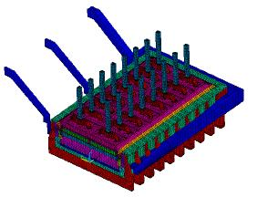
• Has provided to Lauralco the modeling tools (both 3D ANSYS based thermo-electric models and Dyna/Marc cell simulator that helped them become the most efficient smelter of the industry.
